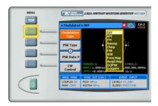
3. Select the **Chirp** modulation type from the list box using the arrow keys, and press **ENTER**.
