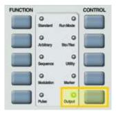
**8.** Define the channels in the **Output** section as being ON or OFF, modifying the settings using the dial or the cursor keys.
